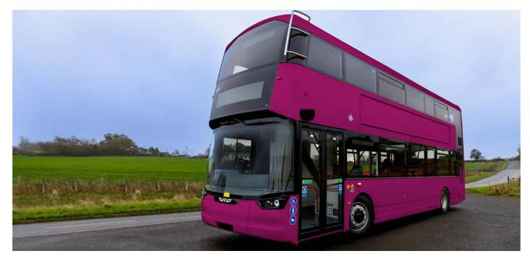
The StreetDeck Ultroliner EU6 is available with two ultra low emission efficient diesel engine choices: the new Cummins 6.7 litre 6 cylinder and the current Mercedes 5.1 litre 4 cylinder engine. Our StreetDeck EU6 Ultroliner and its engine choices remains the UK's favourite. All these buses can be repowered at mid-life to zero-emission BEV technology with NewPower.
